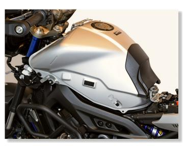
REMOVE THE FUEL TANK. REMOVE THE AIRBOX.
