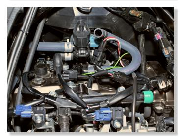
PLUG QSH CONNECTORS IN-LINE WITH THE IGNITION COIL CONNECTORS. (BLACK, 2-POLE CONNECTORS BELLOW AIRBOX)
