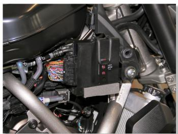
CUT THE WHITE/YELLOW (SPEED SIGNAL) WIRE AT THE ECU CONNECTOR.
