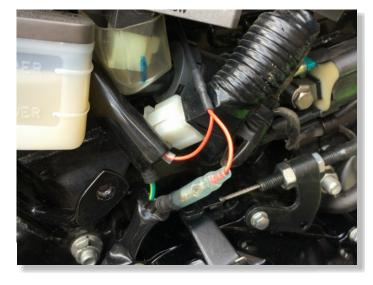
WRAP THE WIRES AND CABLES WITH BLACK TAPE NEATLY.
